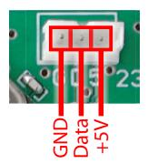
Figure 16: 1-Wire Pinout
