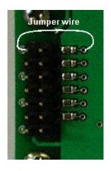
Figure 18: Bypassing 240 ohm Resistor
