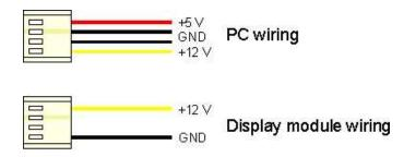
Figure 6: Wiring for 12V Modules
