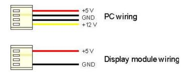
Figure 4: Wiring for 5V Modules
