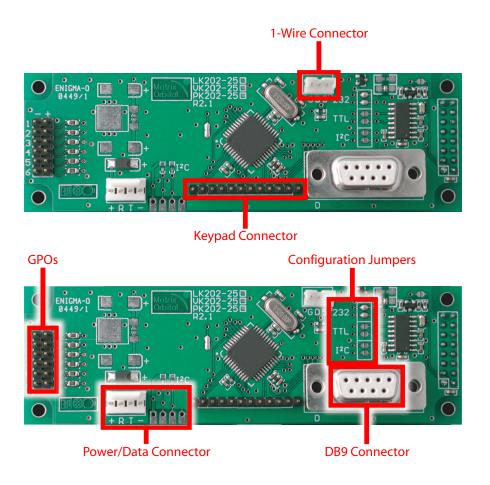
Figure 2: Electrical Connections
