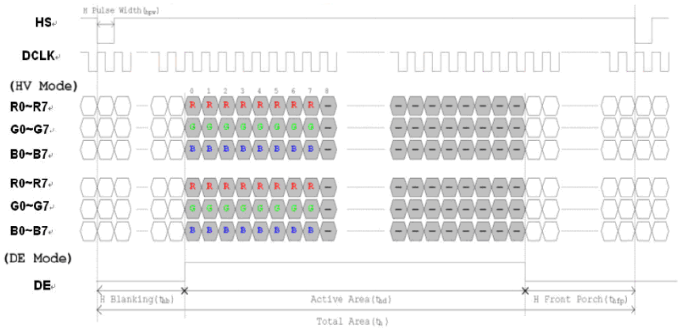
Figure 5: Horizontal Input Timing Diagram
