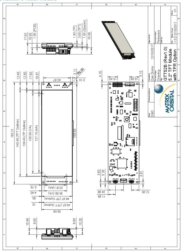
Figure 17: GTT52B-TPR Dimensional Drawing
