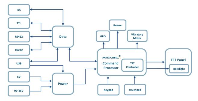
Figure 2: Functional Diagram
