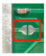
Figure 9: DB-9 Solder Jumper
