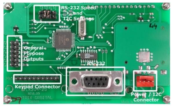
Figure 2-2 Electrical Connections
