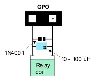
Figure 2-12 Clamping a Relay
