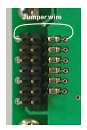
Figure 2-11 Bypassing 240 ohm resistor
