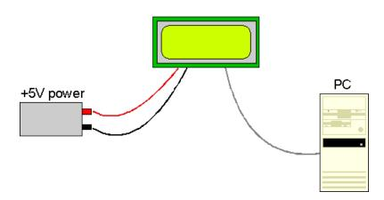
Figure 1-1 Connections for Testing
