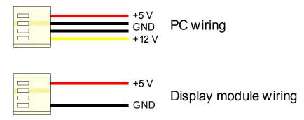
*Figure 2-4 Power Connector wiring differences*
