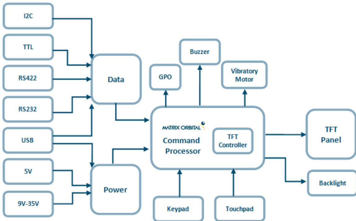
Figure 2: Functional Diagram
